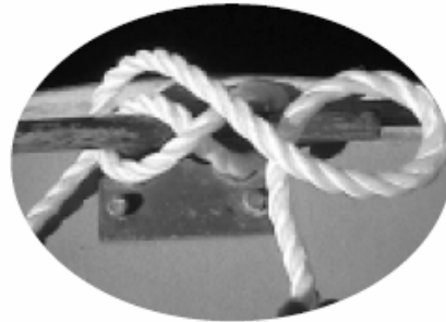
FIGURE EIGHT: To stop end of rope from passing through a cleat, etc.
