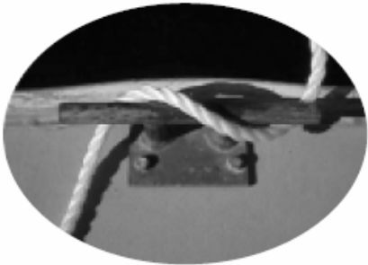
FIGURE EIGHT: To stop end of rope from passing through a cleat, etc.
